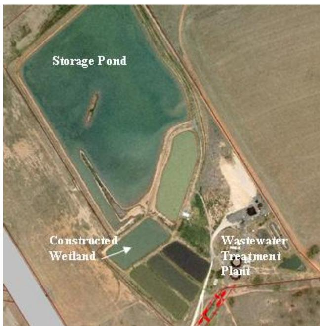
**Figure 1: Junee Wastewater Treatment Plant**
